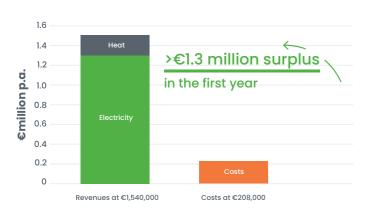
Assuming that the anaerobic digestion of biosolids uses a state-of-the-art grid stabilization method, sewage gas is valued as a cost-neutral energy source. In this scenario, onsite electricity generation with a sewage gas-fired CHP system delivers maximum efficiency and cost-effectiveness by simultaneously using the heat. In ideal circumstances, a CHP system fueled by sewage gas recoups its entire cost in the first year of operation.
